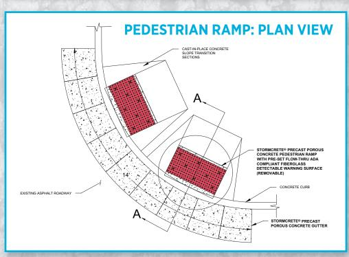
Green Corner™ with Flow-Thru Detectable Warning Surface
