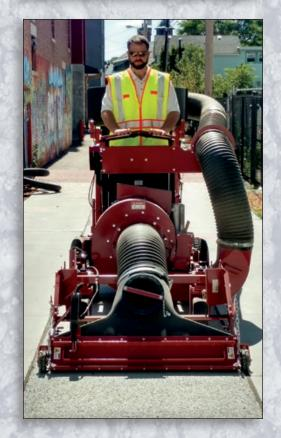
The Stormwater SUV is a ride-on pure-vacuum unit specifically tailored for the porous pavement industry.
