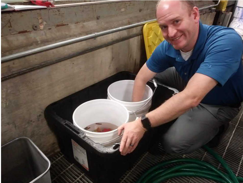
Figure 27. Two bucket rinse method of cleaning sediment from gross solids. The grey mesh wastebasket (lower left) was used to dry gross solids in the oven.
