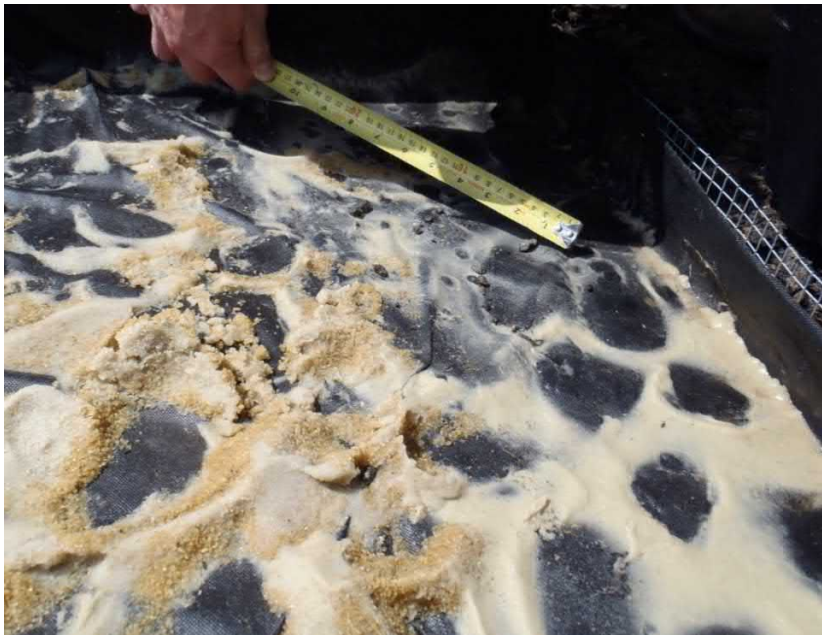
Figure 63. Sediment remaining on geotextile when rocks were removed from RLI.
