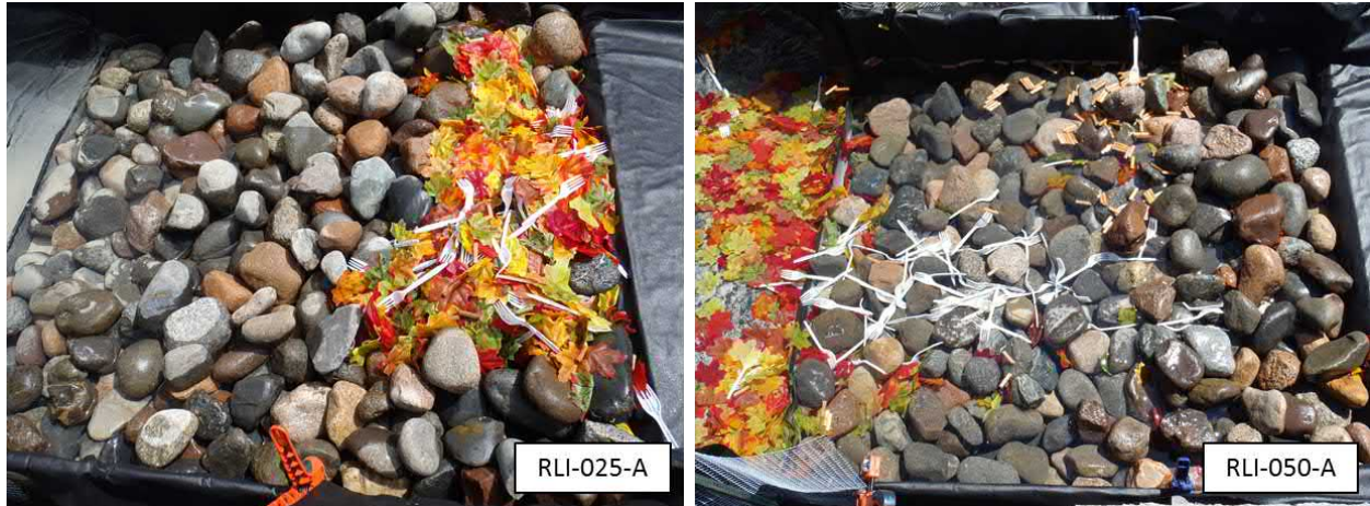
Figure 57. Rock lined inlet after testing at 0.25cfs for 40 minutes (left) and 0.50cfs for 20 minutes (right).
