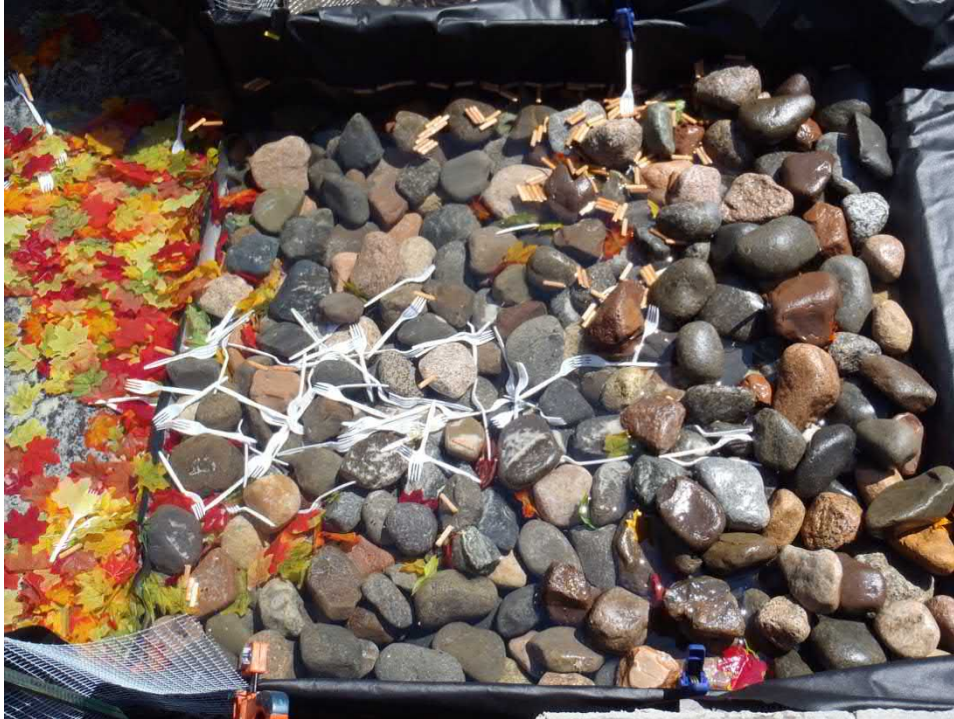
Figure 12. Rock lined inlet after testing at 0.50 cfs for 20 minutes. Entrance from the curb cut comes into the RLI from the right of the picture; exit into the bioretention practice at left.
