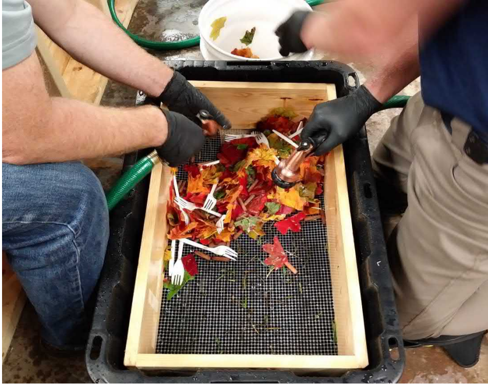
Figure 25: Rinsing gross solids on a mesh box over a watertight bin. This method was later revised (see Figure 27).
