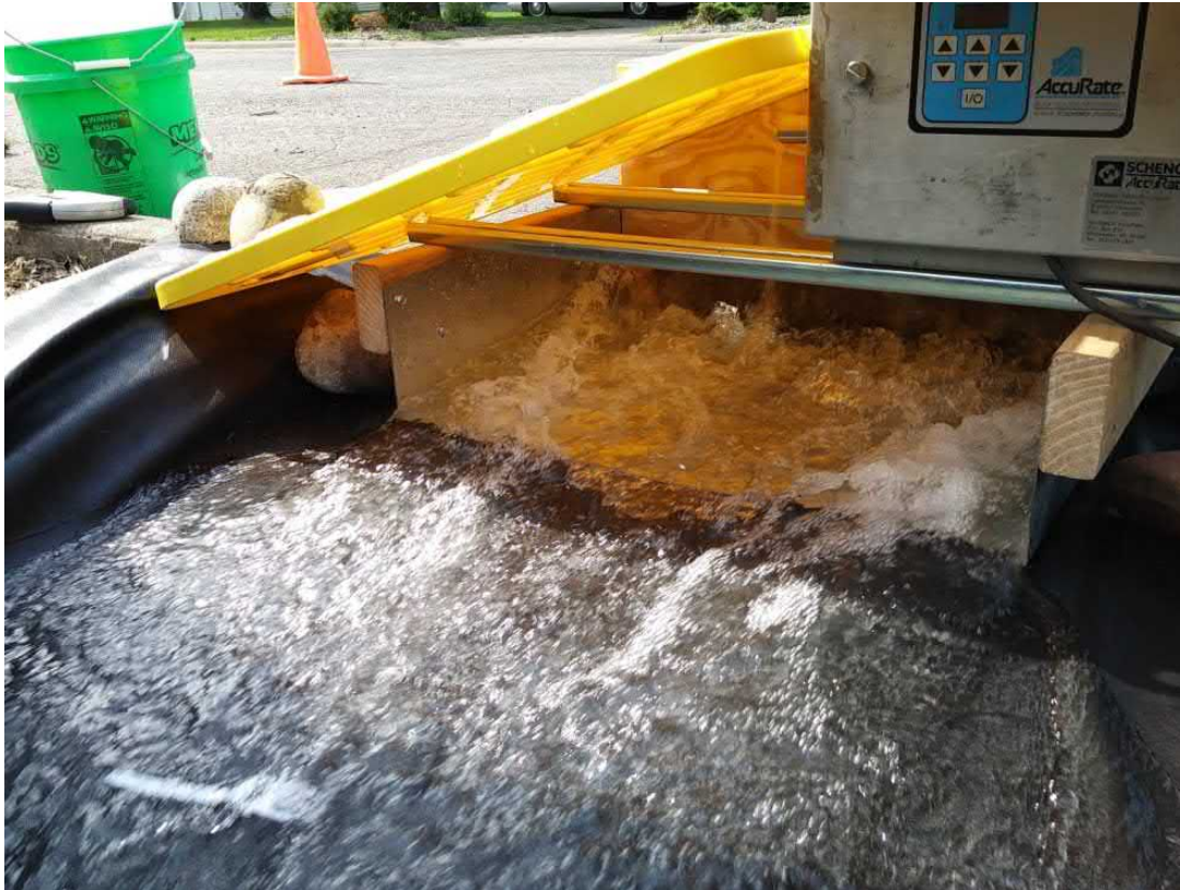
Figure 22. Sediment feeder and flow distributor.
