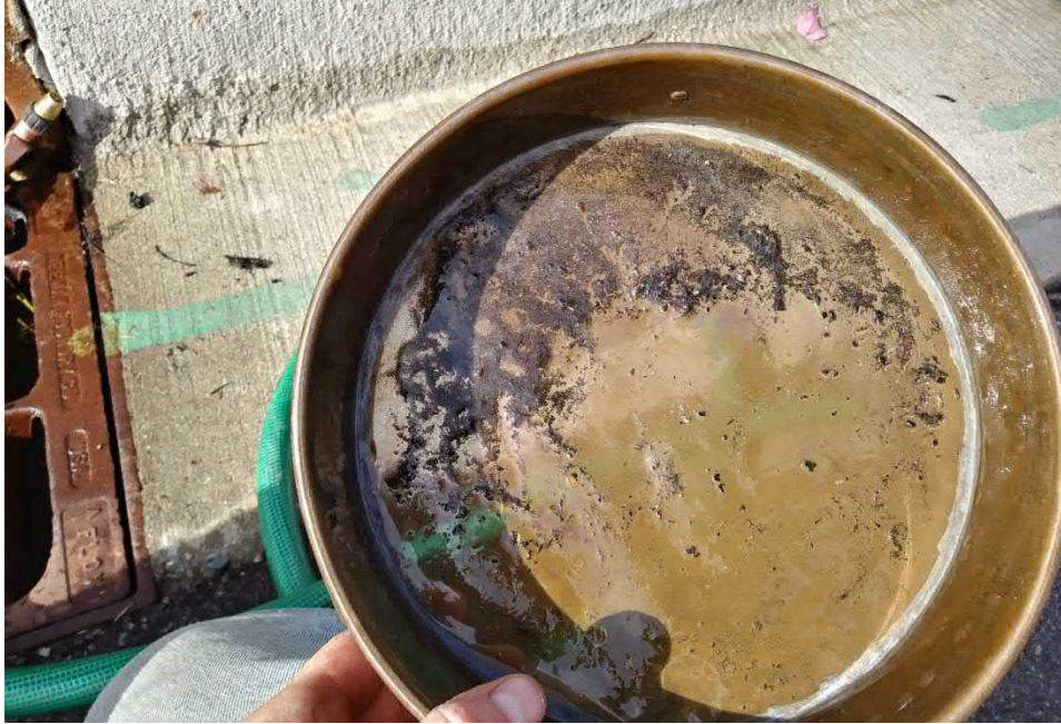
Figure 47. Fine organic material retained on sieve.
