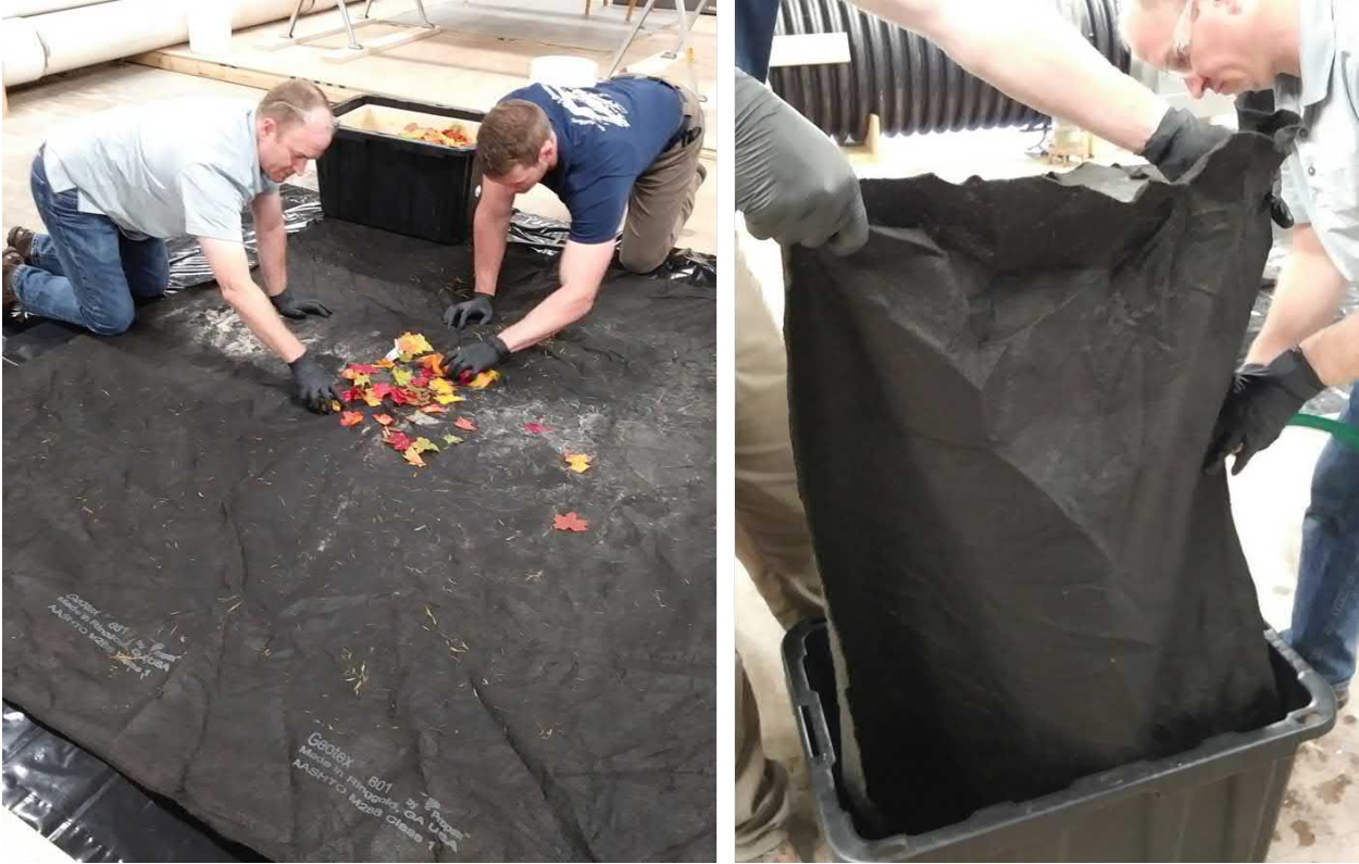
Figure 34. For the grass lined inlet, solids passing the pretreatment and landing in the geotextile were processed and weighed. Gross solids were removed from the geotextile at SAFL (left) and sediment was rinsed from the fabric (right).
