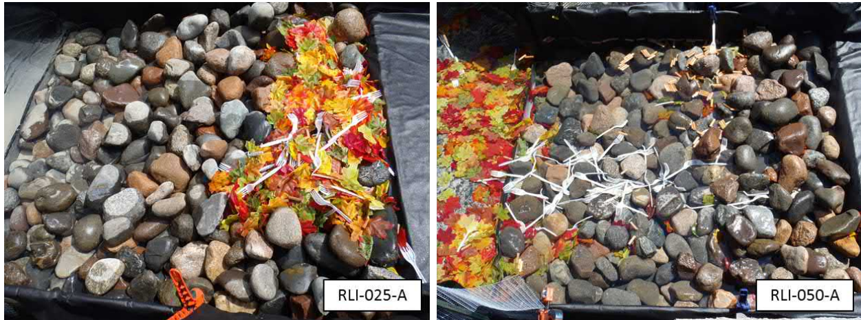
Figure 62. Rock lined inlet after testing at 0.25 cfs for 40 minutes (left) and 0.50 cfs for 20 minutes (right).
