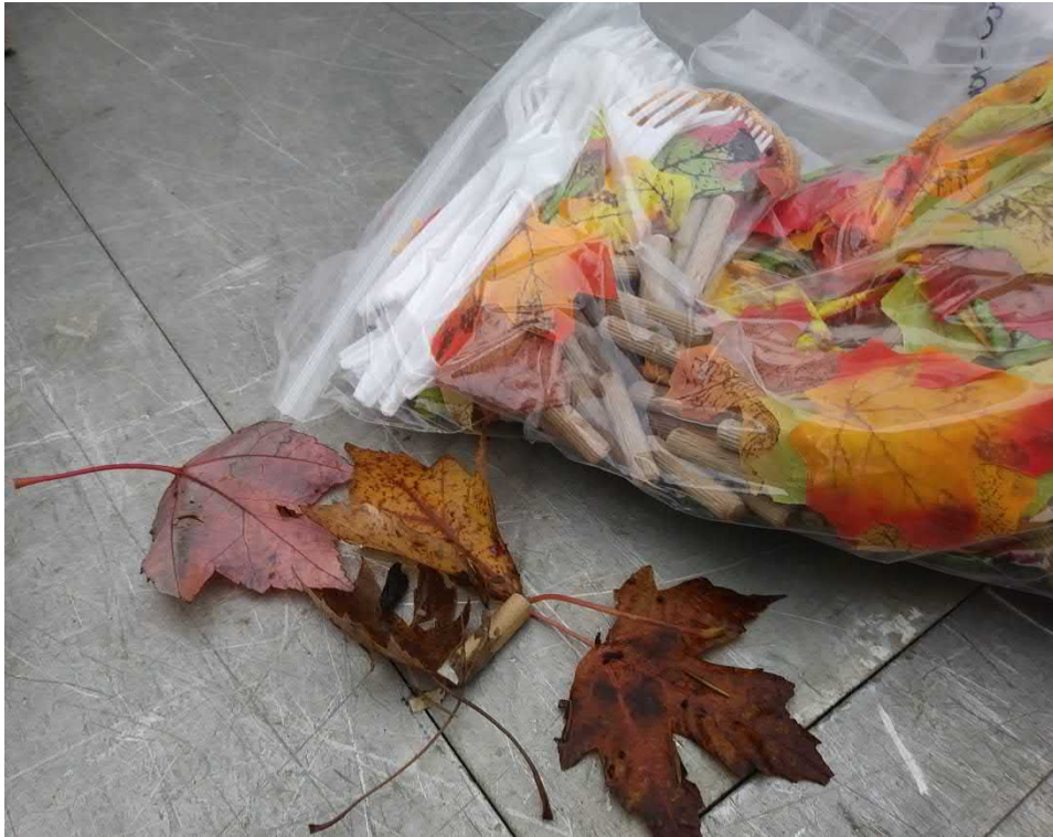
Figure 16. A bag of synthetic gross solids used in testing (leaves, dowels, and forks) next to actual maple leaves and a cigarette butt recovered from the Bloomington site.
